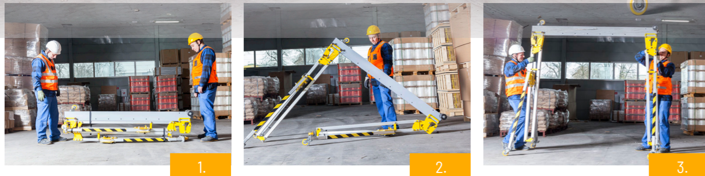
FSB - Crane unfolding sequence
